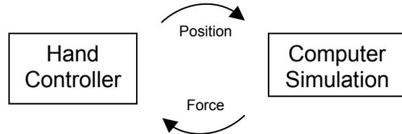
**Device Latency:** The time delay between sending a command to a device and receiving a response from that device. This would normally include geometrical computations (the forward and inverse kinematics), some of which may take place in the computer.
