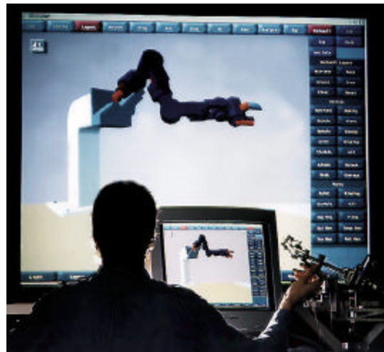
Figure 4: Operator working with a virtual model of a remote robot.
